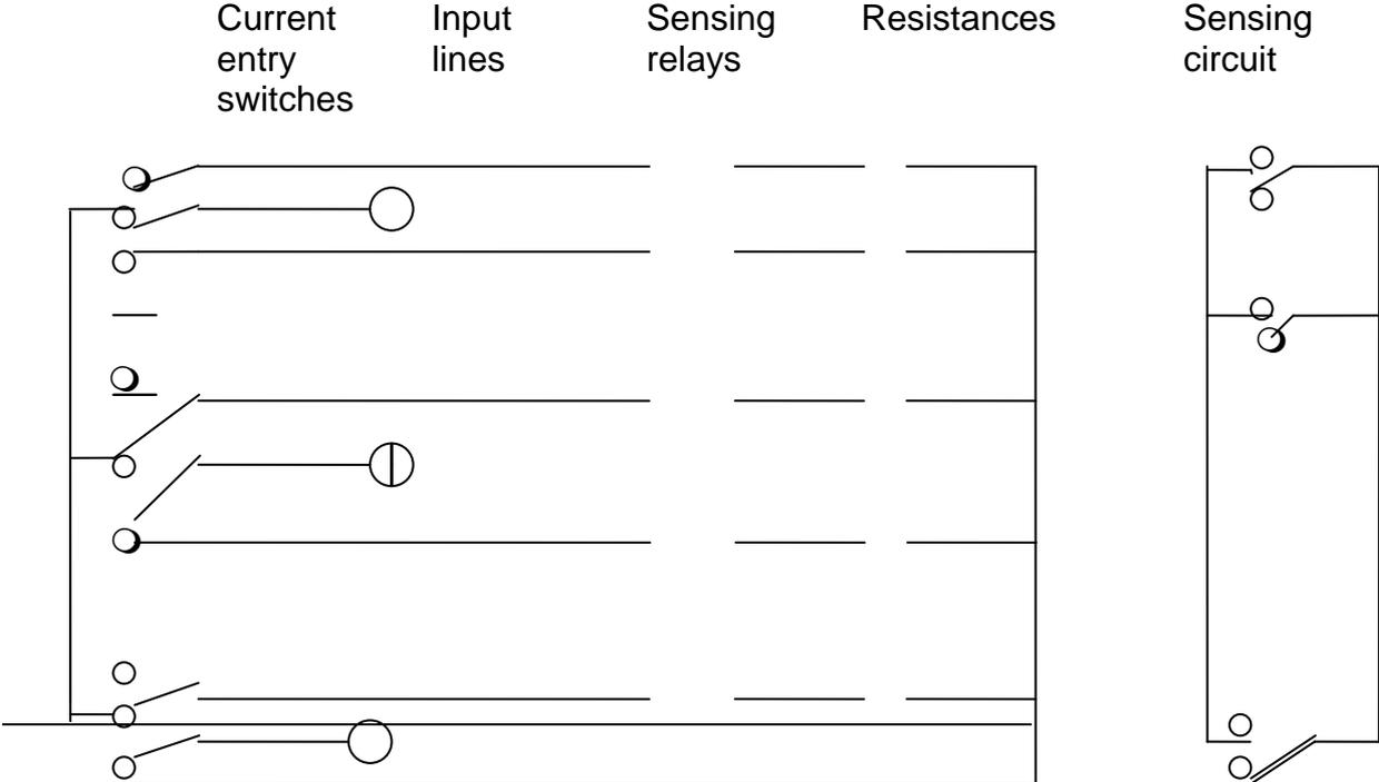
Each sensing relay has two windings, in opposite directions, and the relay is “up”, i.e. the relay switches operate, when current passes through one coil but not through the other. When current passes through both coils or through neither coil the switches do not operate, and the relay is in its normal or “down” position. The negative terminals of both coils are connected to the negative side of the main spider circuit, shown by the green line in the
